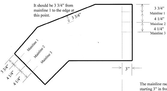
The mainline radius is measured exactly at the end of the 20" end. There is no easement on this end.
